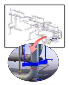
Figure 1. Typical hanger design and location.
