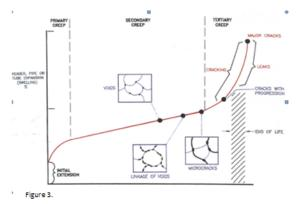
Stages of Creep Development. As creep stages progress, illustrated in the graphic above, the voids begin to link with one another, developing into cracks which then propagate through the material eventually causing leaks or failures.
