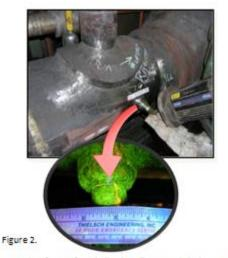
Example of a surface indication discovered during a routine outage inspection.
