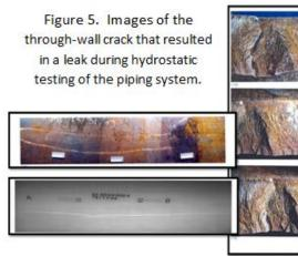
The results of the metallurgical evaluation confirmed that the pipe segment had been subject to localized overheating. The localized overheating was sufficiently severe to result in reaustenitization, grain growth and cracking. The cracking and microstructural transformations introduced during the localized overheating rendered the pipe subject to brittle failure during subsequent handling.
